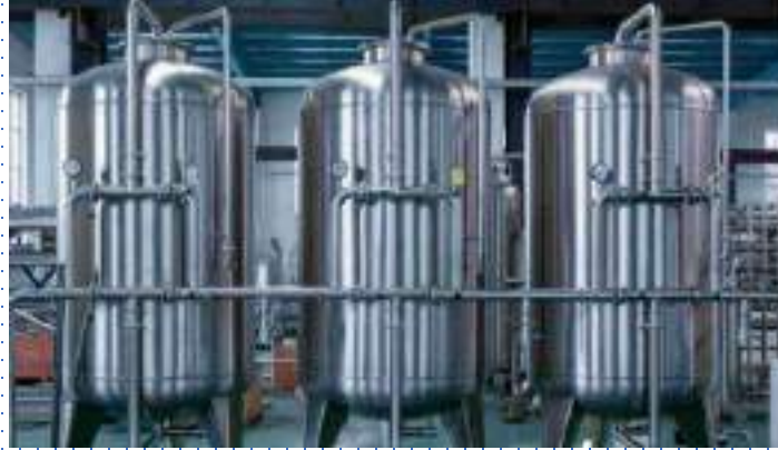
Filter system for mechanical water purification
